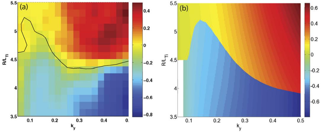
**Figure 7.** (a) Averaged nonlinear frequency  $\bar{\omega}$  (colour coded), the  $\bar{\omega} = 0$  contour line (black) may be used to mark the TEM–ITG transition. (b) The corresponding frequencies of the dominant linear microinstability.
