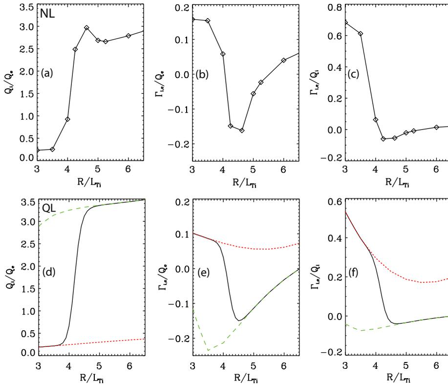
**Figure 12.** The black curves depict the nonlinear (top) and quasilinear (bottom) ratios of the different fluxes for  $R/L_n = 2.5$ . The dotted and dashed curves correspond to the values of the underlying TEM and ITG modes, respectively.
