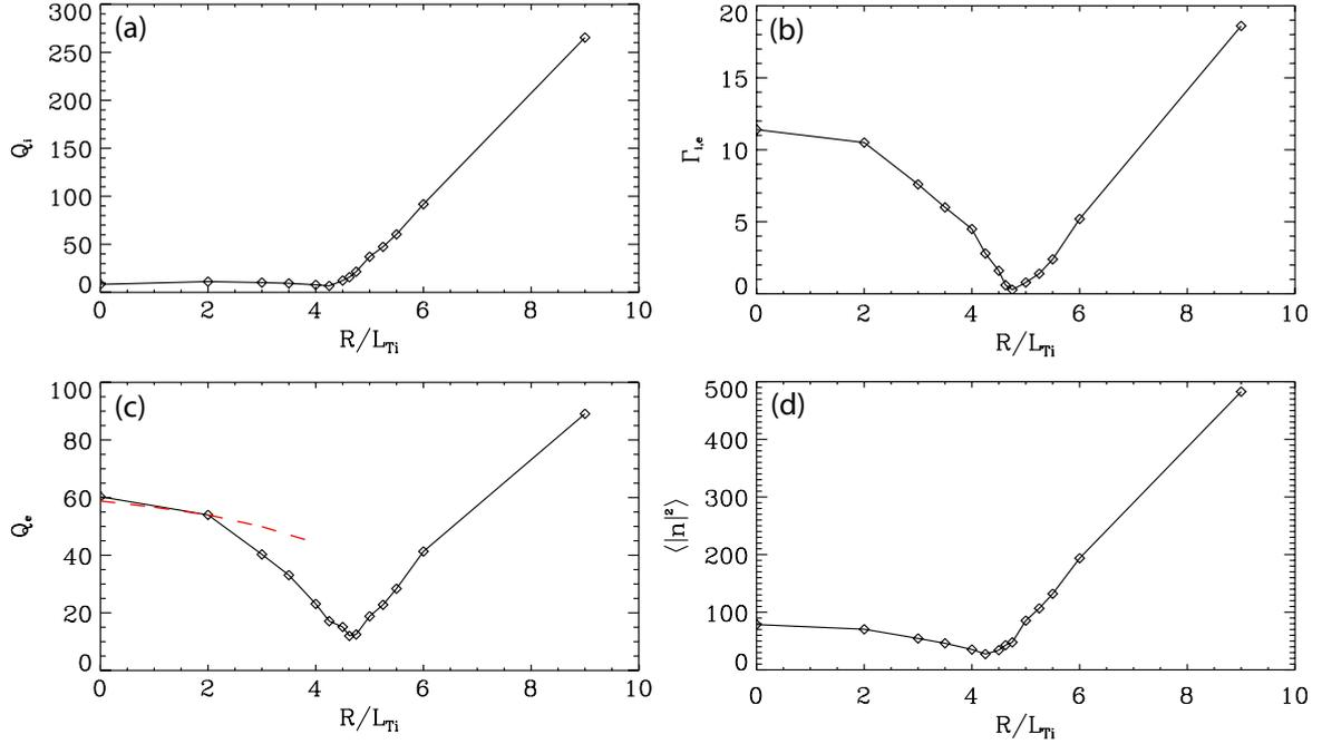
**Figure 1.** Ion and electron heat (a), (c) and particle (b) fluxes and the fluctuation level (d) as a function of the ITG. The dashed curve in (c) corresponds to the TEM transport model described in [6].
