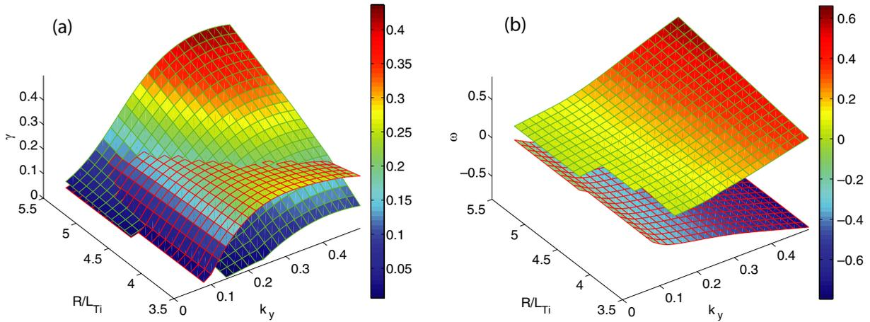
**Figure 4.** Linear growth rates (a) and frequencies (b) as a function of  $k_y$  and  $R/L_{Ti}$ . The TEM and ITG modes are distinguishable by the dark and light (red and green) colour of the mesh, respectively. The missing patch at low  $k_y$  and  $R/L_{Ti}$  is due to the stability of the ITG mode for these parameter values.
