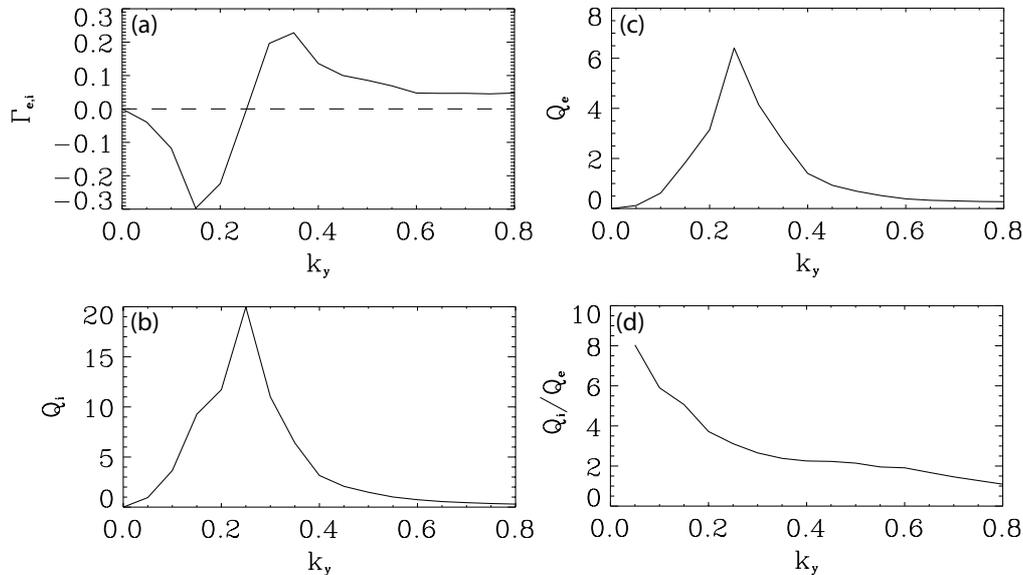
**Figure 13.** Spectra of the particle flux (a), the ion and electron heat fluxes (b), (c) and the ratio of the ion and electron heat fluxes (d) close to the second zero-crossing of the particle flux for  $R/L_n = 2.5$  and  $R/L_{T_i} = 6.0$ . The dashed line in (a) corresponds to  $\Gamma = 0$ .
