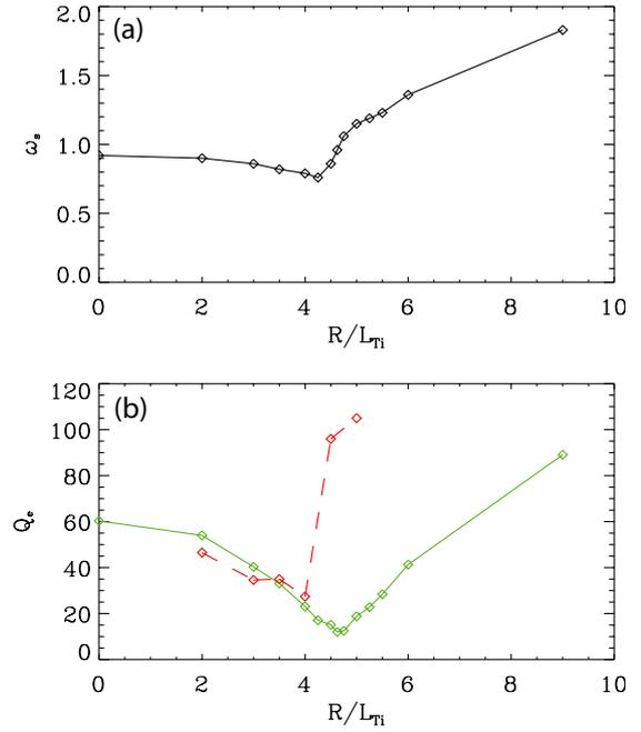
**Figure 3.** Shearing rate  $\omega_s$  (a) and electron heat flux  $Q_e$  (b) as a function of  $R/L_{Ti}$ . Continuous lines correspond to full nonlinear simulations, for the dashed curve, the zonal flows have been artificially suppressed.
