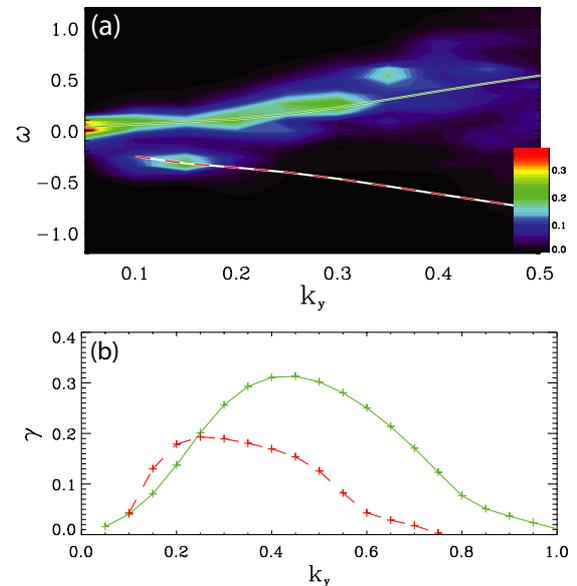
**Figure 5.** (a) Normalized nonlinear frequency spectrum (colour coded) as function of  $k_y$  for  $R/L_{Ti} = 4.625$ ; the dashed (red) and continuous (green) lines are the linear frequencies for TEM and ITG modes respectively. (b) The corresponding linear growth rates.
