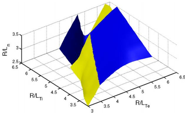
**Figure 10.** The  $\Gamma \approx 0$  surface (dark/blue shading) as predicted by the quasilinear model defined in section 4, and the ITG-TEM transition surface (light/yellow shading) for the ‘typical’  $k_y = 0.25$  mode. The region with the particle pinch is ‘behind’ the blue surface in this view.
