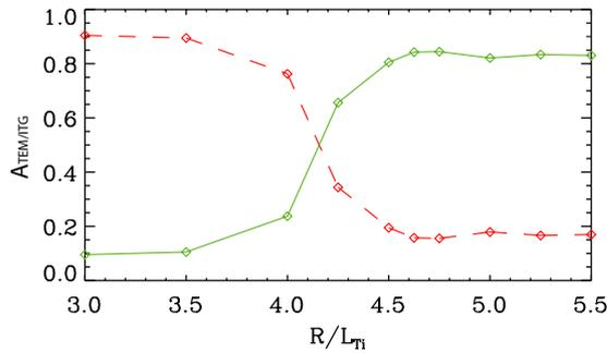
**Figure 6.** Normalized TEM (dashed line) and ITG (continuous line) contributions as defined in equation (1) as a function of  $R/L_{Ti}$ .
