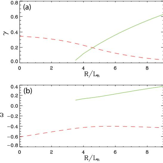
**Figure 2.** The linear growth rates  $\gamma$  (a) and frequencies  $\omega$  (b) of the TEM (dashed) and ITG mode for a ‘characteristic’ wavelength of  $k_y = 0.25$ . The modes are clearly distinguishable by the sign of their frequency over the full parameter range.
