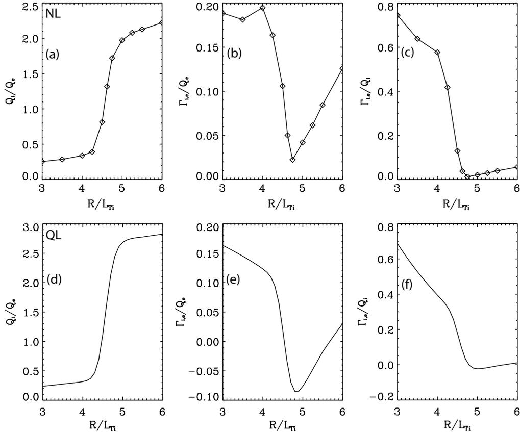
**Figure 9.** Nonlinear flux ratios (top) versus quasilinear flux ratios (bottom) as defined by equation (2).
