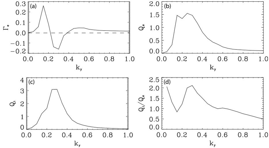
**Figure 8.** Particle flux (a), electron and ion heat fluxes (b), (c) and the ratio of the ion and electron heat fluxes (d) as a function of  $k_y$  for  $R/L_{Ti} = 4.625$ . The dashed line in (a) corresponds to  $\Gamma = 0$ .
