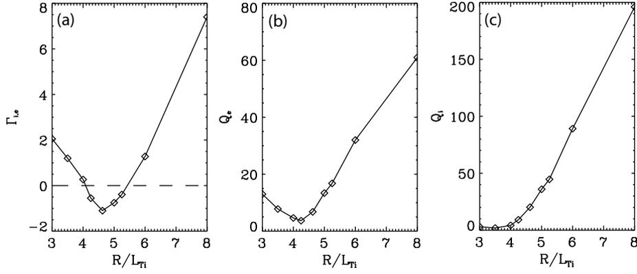
**Figure 11.** The particle flux (a) and the electron and ion heat fluxes (b), (c) for the reduced density gradient  $R/L_n = 2.5$ , showing a particle pinch for  $R/L_{Ti}$  between 4.1 and 5.5. The dashed line corresponds to  $\Gamma = 0$ .
