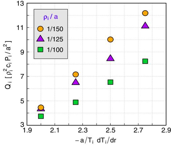
FIG. 2 (color online). Ion-heat-flux scaling for different  $\rho^*$  values from flux-surface GENE simulations. Here  $P_i$  is the ion pressure,  $a$  is the minor radius of the torus,  $r$  denotes the radial coordinate,  $c_i$  is the ion sound speed, and  $\rho_i$  is the ion gyroradius.
