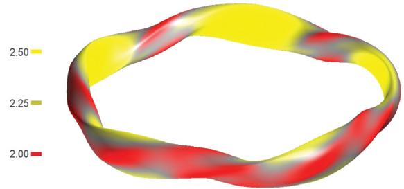
FIG. 3 (color). The turbulence-optimized MPX stellarator design. Shown is the magnetic field strength (tesla) over a magnetic surface. MPX is the first example of a quasisymmetric stellarator, similar to W7-X, but with reduced turbulent transport. For this proof-of-principle configuration no attempt has been made to minimize the bootstrap current (which, however, takes acceptable values) or the alpha-particle losses.
