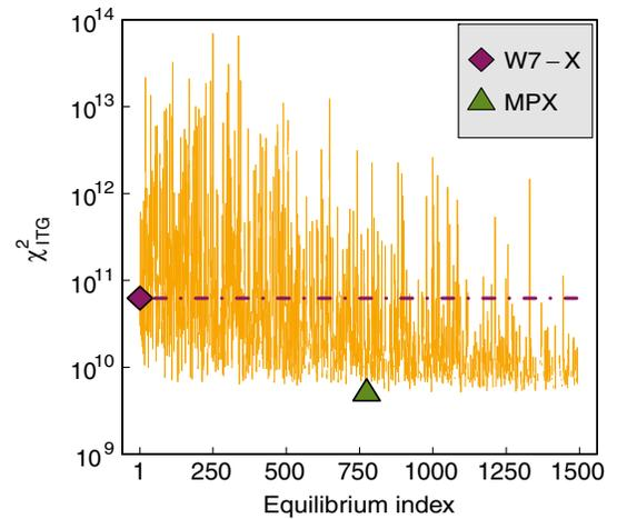
FIG. 4 (color online). The MPX configuration was produced during a STELOPT run equipped with the Differential Evolution algorithm. The fluctuations in the cost function represent the stochastic evolution of the population and diminish as the algorithm converges. MPX was singled out before the collisional transport (not shown here) started to increase.
